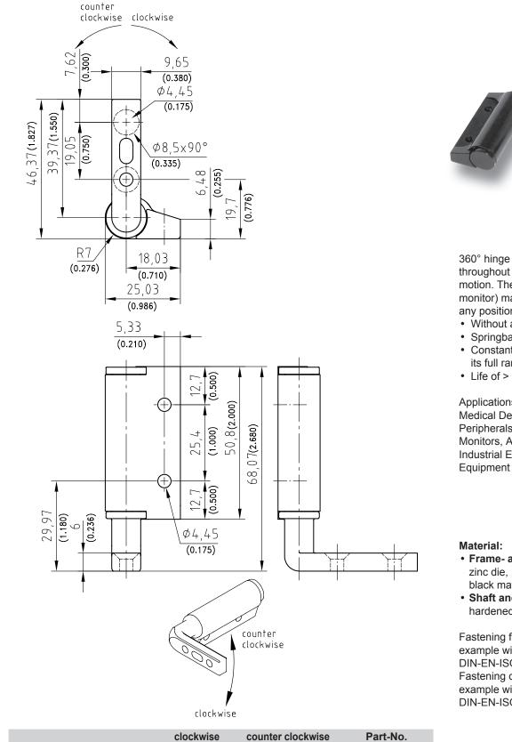
360° hinge with constant torque throughout its full range of motion. The object ( door, monitor) may be moved into any position and with remain.
